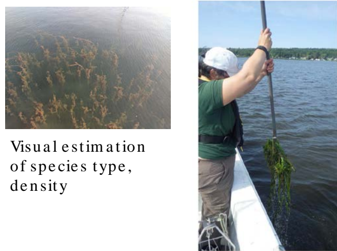
Figure 3.7. Rake twist sample immediately after retrieval from the water from an area with dense SAV, undergoing visual estimation of density.
