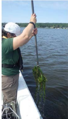
Figure 3.7. Rake twist sample immediately after retrieval from the water from an area with dense SAV, undergoing visual estimation of density.
