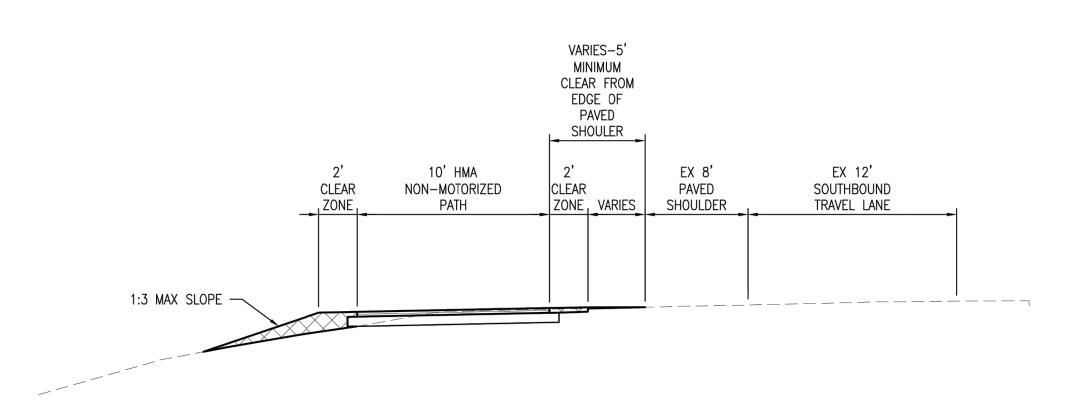
MAPLE ST. TO OLD ALLEGAN ST. PROPOSED 10' HMA NON-MOTORIZED PATH TYPICAL SECTION FROM 350' NORTH OF MAPLE ST. TO 275' SOUTH OF OLD ALLEGAN ST.
