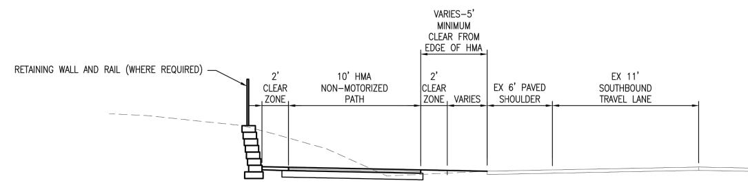
LAKE ST. TO MAPLE ST. PROPOSED 10' HMA NON-MOTORIZED PATH WITH RETAINING WALL TYPICAL SECTION FROM 200' SOUTH OF MAPLE ST TO MAPLE ST
