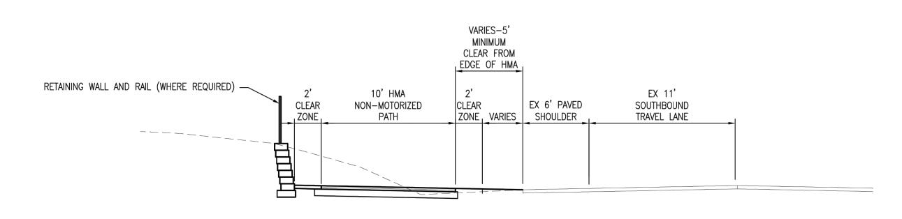
MAPLE ST. TO OLD ALLEGAN ST. PROPOSED 10' HMA NON-MOTORIZED PATH WITH RETAINING WALL TYPICAL SECTION FROM MAPLE ST TO 350' NORTH
