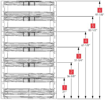
Simply select the number of modules to determine the assembled well height.
